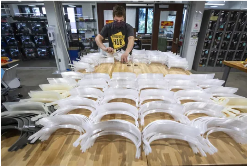
Richard Ensor, sculpture lab manager with the FSU Department of Art, performs finishing refinements on the face shield brackets after they are printed at the Innovation Hub on Florida State University's campus. (Photo: Bruce Palmer/ FSU Photography Services)
