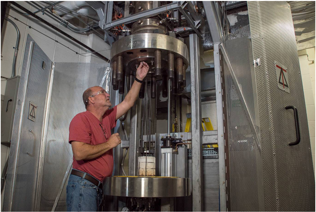
Research Engineer Charles Lamar English works on a specialized furnace used to develop magnet coils from the high-temperature superconductor Bi-2212, a version of bismuth strontium calcium copper oxide. Photo by Stephen Bilenky/National MagLab.
